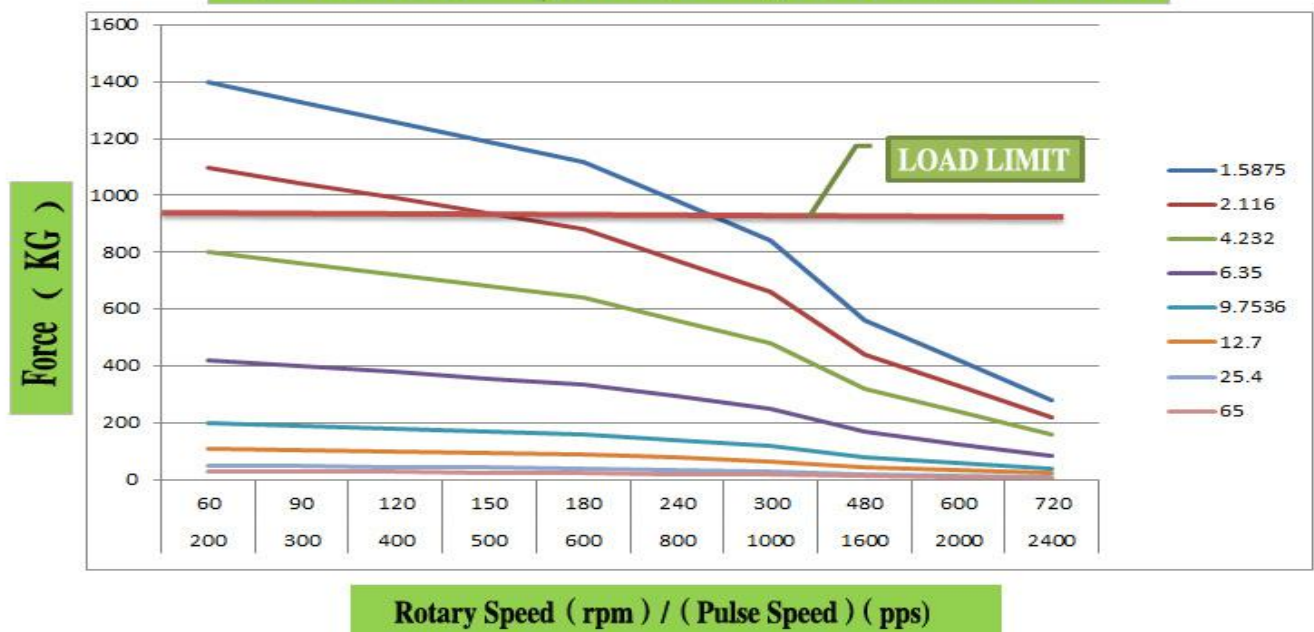
57 SERIES MOTOR LENGTH ( 45mm),24VDC CHOPPER DRIVER
