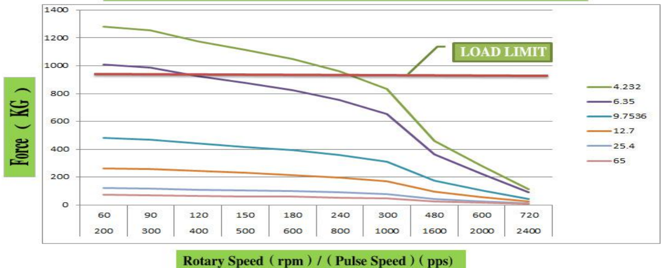
57 SERIES MOTOR LENGTH ( 65mm),24VDC CHOPPER DRIVER
